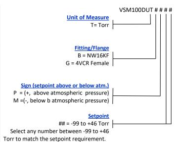
Example: VSM100DUTGP40 (Differential vacuum switch, Torr, 4VCR fitting, setpoint 40 Torr above atmospheric pressure)
