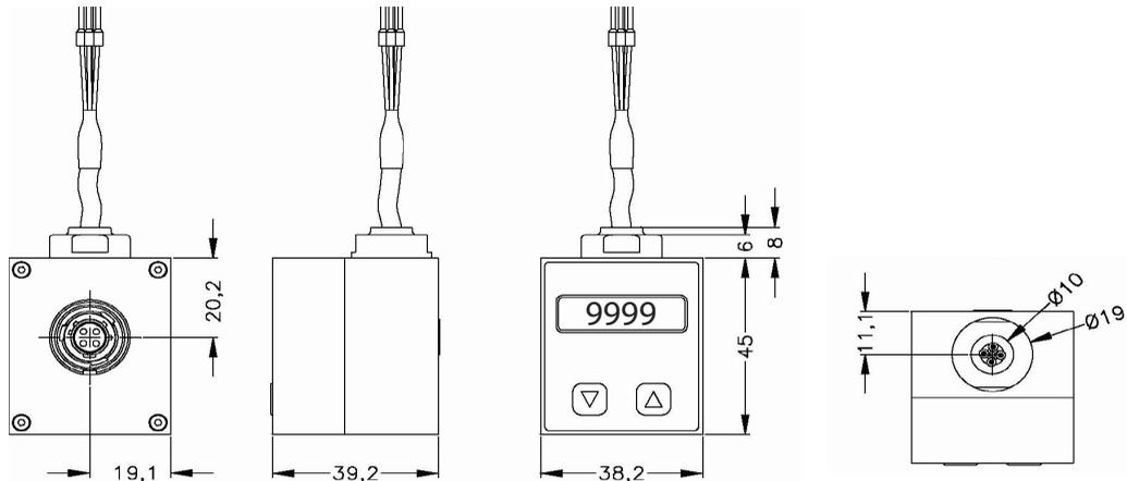
The SolidSense II pressure transducer is available with an optional display: Model LR056, for details on this display see [DS-PR-LR056-eng](#)
