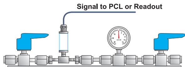
**SolidSense II Pressure Transducer (T4)** has a fully swept path which greatly reduces contamination and eliminates the need for cleaning solvents and disassembly.
